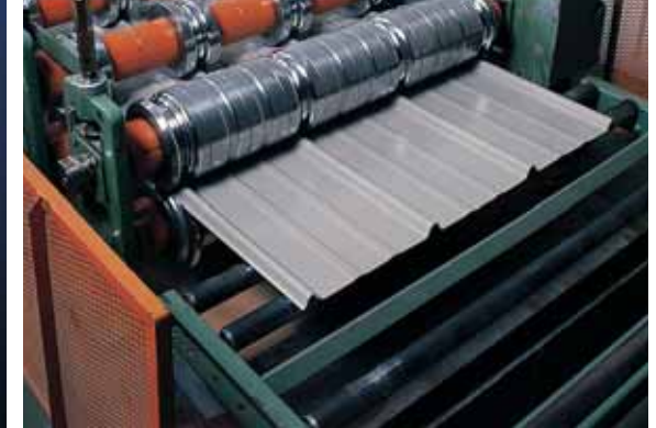
Morton's Steel Roll-Forming Machine
